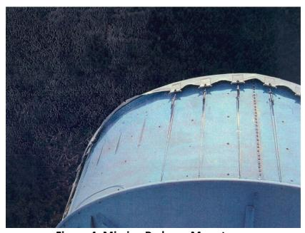
**Figure 4: Missing Radome Mounts**
